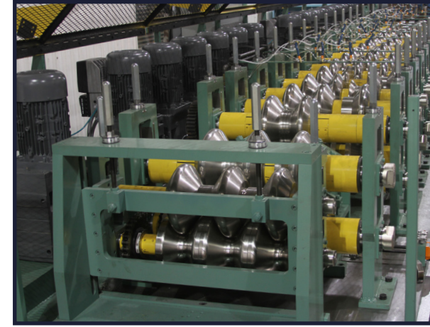
Heavy Gauge Guardrail Line with Torque Vectoring™ Drive System
