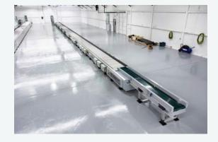
The unique design of our upper rail offers a dedicated raceway for controls and network cabling. This feature significantly reduces installation time and cost.
