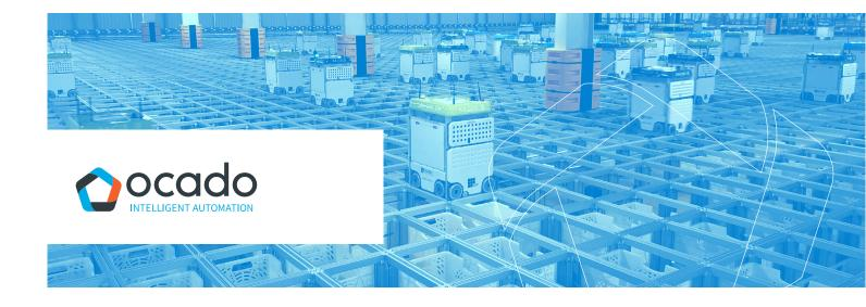
The Ocado Intelligent Automation ASRS is a highdensity cubic storage & retrieval system that combines world-proven automation with AI-powered business intelligence.
