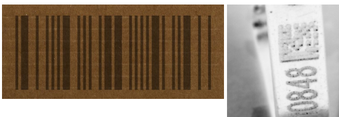
Figure 2: Dark barcodes printed on dark backgrounds (like this 1D barcode on cardboard), or light symbols marked on light or reflective materials (like this 2D Data Matrix on metal), can cause no read results due to poor contrast between light and dark symbol elements.
