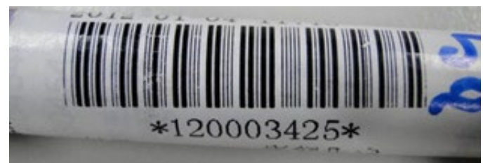
Figure 4: Poor distribution of ink on this test tube barcode label has resulted in some white spots within the bar elements, which may lead to readability issues.
