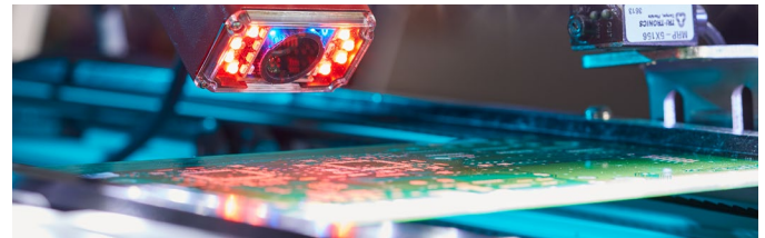
Figure 10: A high-performance imager uses special algorithms to read codes with limited quiet zones, such as a Data Matrix on this crowded PCB.
