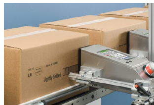
Figure 12: Ink-based case coding equipment prints linear barcodes directly onto cardboard packaging. Movement of products during printing and variations in product speed can greatly impact the quality of these barcodes at the time they are applied.
