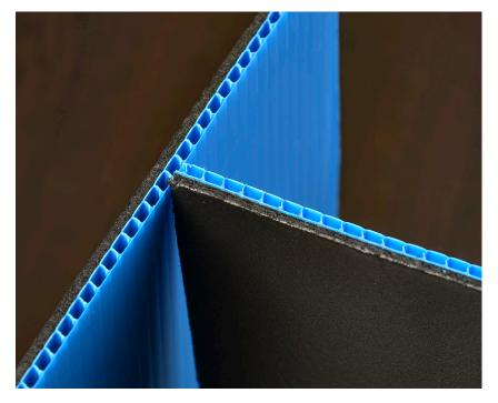
Coroplast<sup>®</sup> cross-linked laminated foam provides a combination of abrasion protection and extra cushioning protection for class "A" packaging applications.
