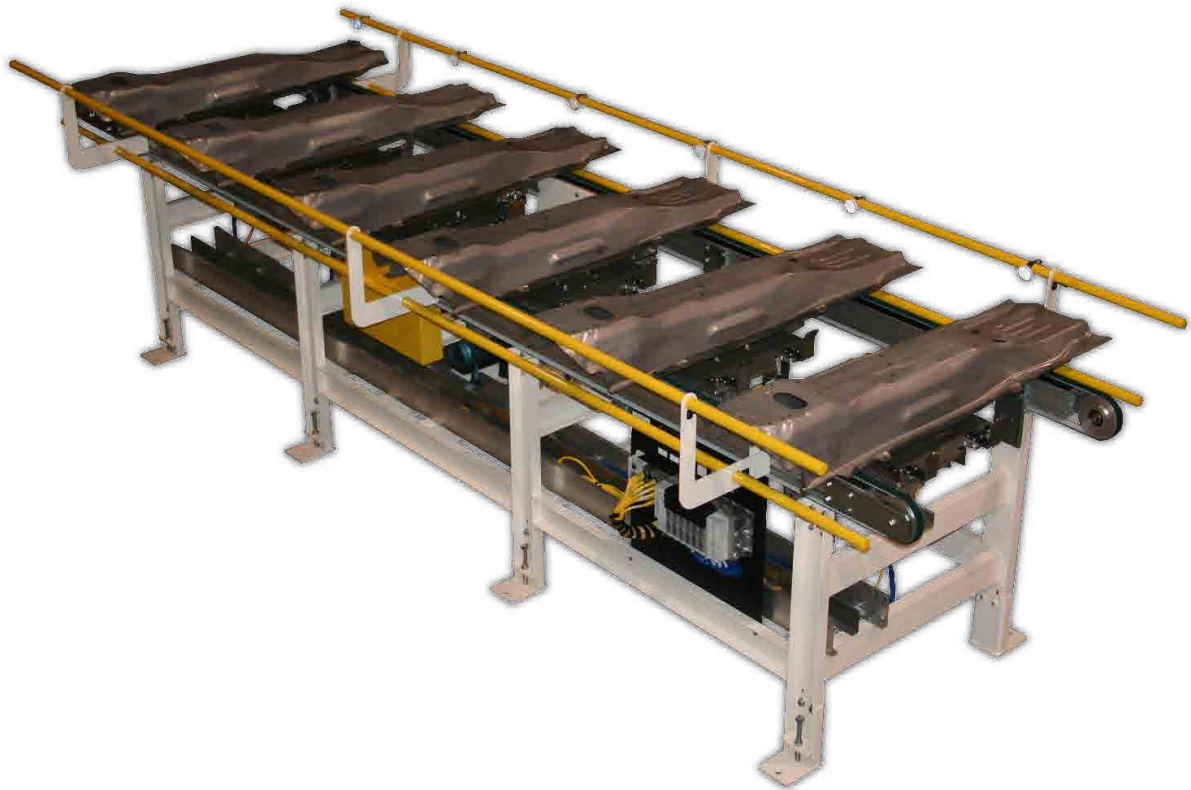
Cast Aluminum Accumulating Conveyor for Robotic Place and Operator Pick
