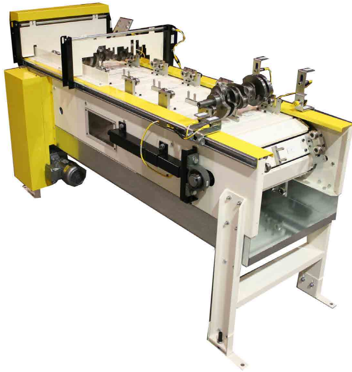
Glass Handling Conveyor With Lift and Center Feature for Solar Panel Industry
