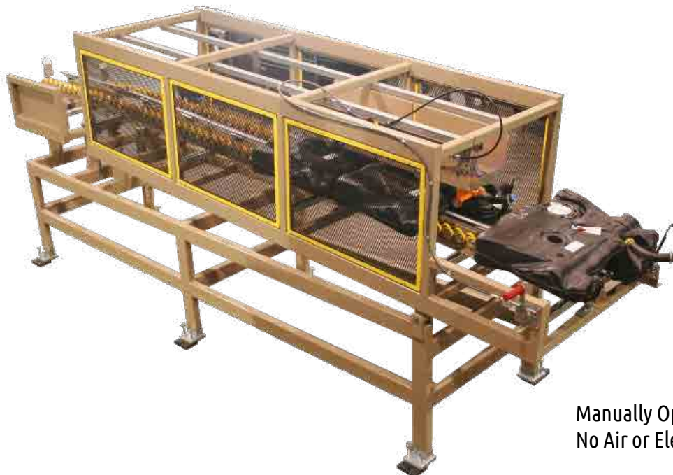
Manually Fed Gravity Conveyor Delivering Gas Tanks to an Assembly Line
