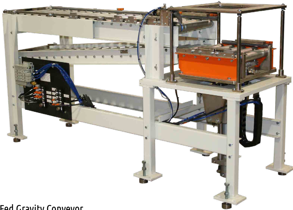
Manually Fed Gravity Conveyor Delivering Gas Tanks to an Assembly Line
