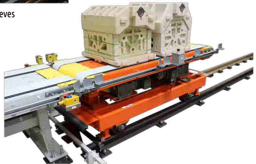
Sand Core Assembly Timing Belt Conveyors with Powered Cart
