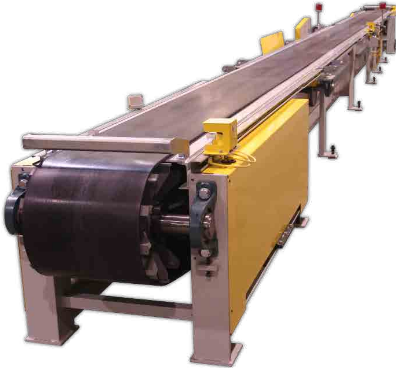
Extra Heavy Duty Belt Conveyor For Foundry Application
