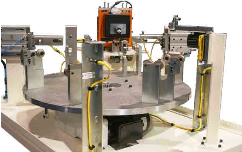
Telesis Part Marking Dial Table with Vision Inspection
