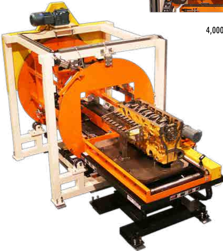
Rotates Palletized Cast Engine Block 90° for Inspection
