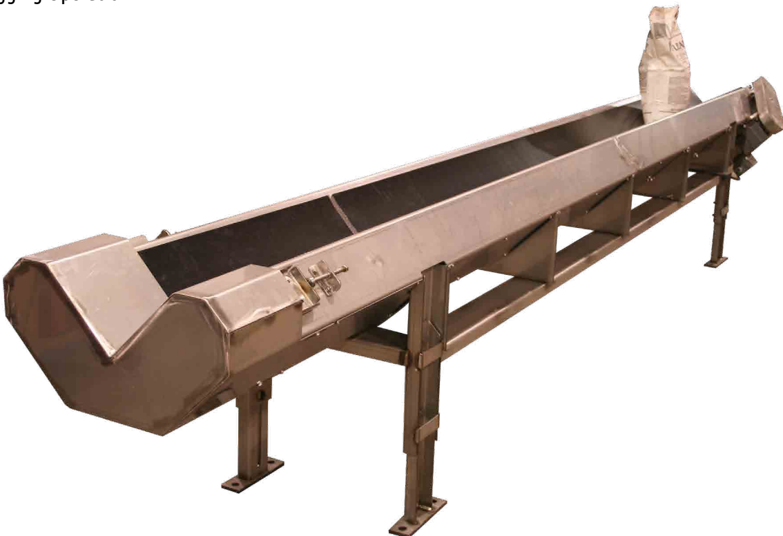
Stainless Steel V- Trough Belt Conveyor For Bagging Operation
