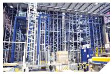
The automatic systems with stacker crane for pallets are automatic storage systems that use robotic equipment for the handling of loads.
