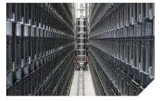
The miniload system uses robotic equipment for the direct handling of plastic boxes or trays.
