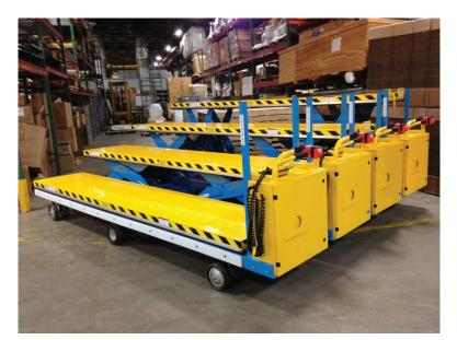
A window and door manufacturer recently improved efficiency and ergonomics in its manufacturing facility by using long, motorized lift table carts as part of an innovative material handling and production solution. The project not only utilized custom motorized carts, but also modified material handling methods to create safer, more efficient parts processing.
