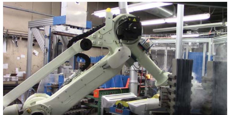
The robot places battery lugs in molten lead.
