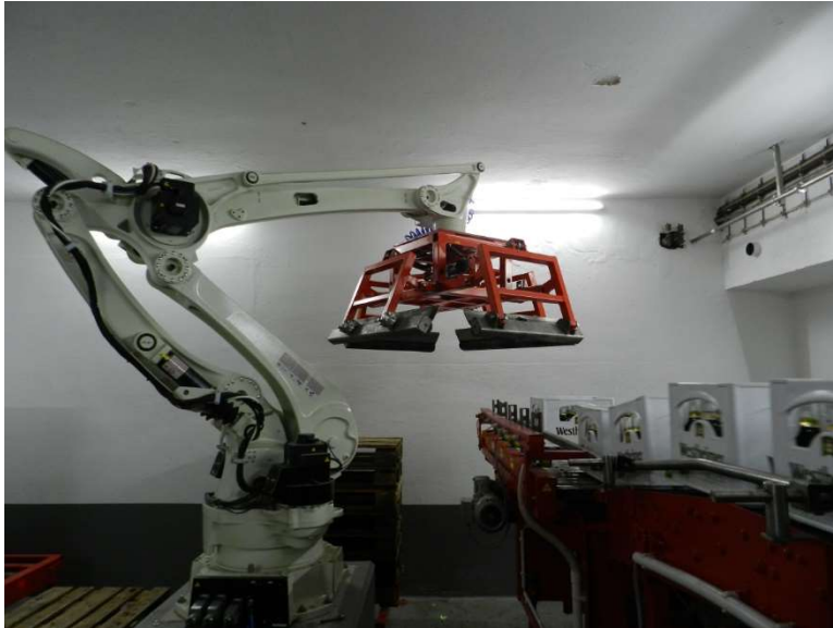
The Kawasaki robot CP500L processes more than 1,200 crates per hour.
