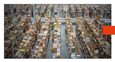
On racking, a standard pick is a minimum of a 16 ft round trip and picking from the furthest point would be a 65 ft round trip.
