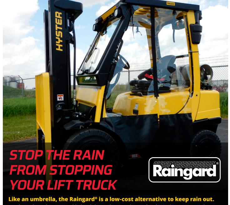
Sturdy steel panels are assembled and clamped to a truck's overhead guard, mounting easily without special tools.
