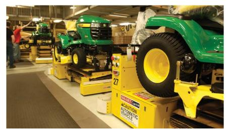
had been using a fleet of over 50 wire-guided AGVs to manufacture several generations of John Deere lawn tractors for about 20 years. Now that they had been in service beyond their normal life span, the additional costs of maintenance and the steep price of newer replacement units caused Deere analysts to investigate SmartCart technology as an alternative.
