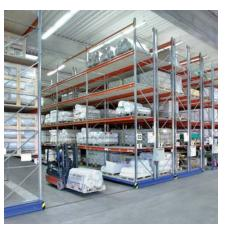
META cantilever racks are the suitable solution for storing all kinds of long goods horizontally or vertically, and for storing sheet goods and panels.
