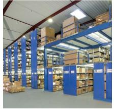
META shelving systems – are built using just two basic components (frame and shelf) and complemented with an extensive range of available accesories. This allows to create either single shelf rows or complex systems for all types of small parts storage applications.
