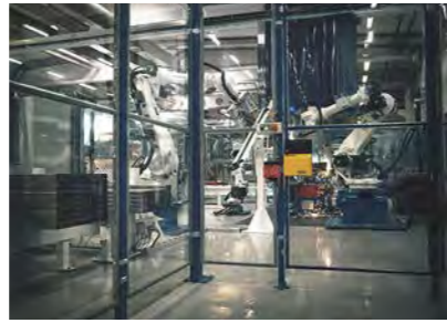
POLYCARBONATE PANELS Gives good overview and protects against fluids and small particles.
