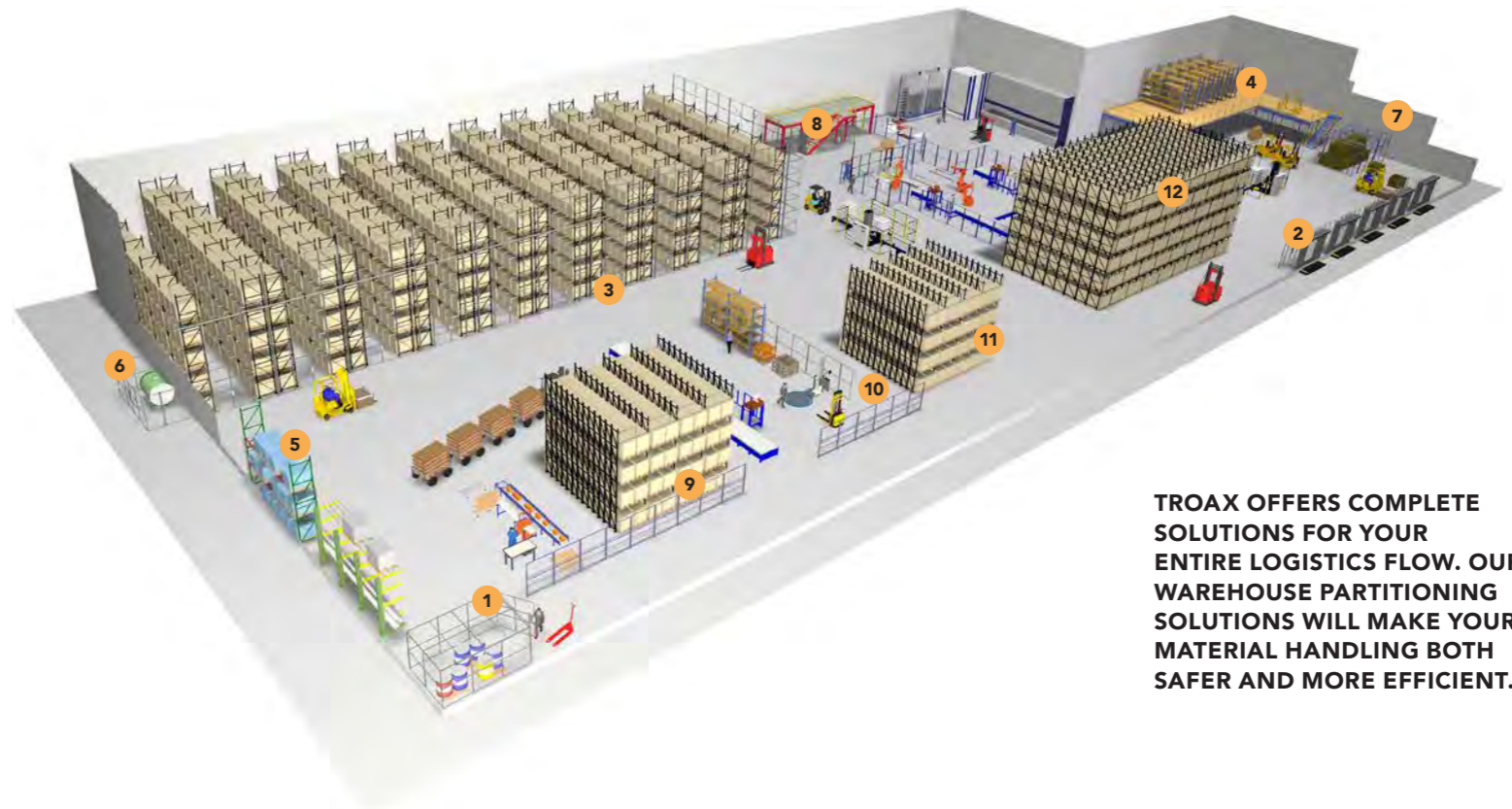
4 MEZZANINE GUARD The Mezzanine system with posts, panels, kick plates and guard rail protects both people and loose objects from falling down.
