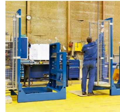
Mechanical assembly of the lifting unit
