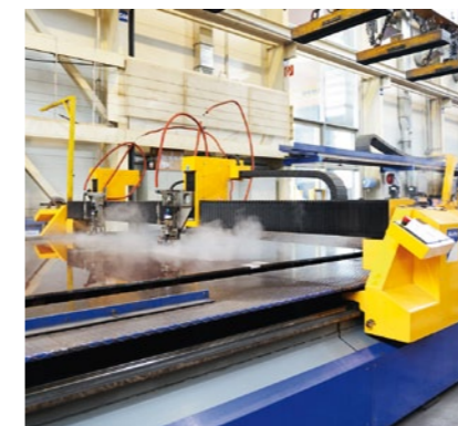
Marking and drilling facility
