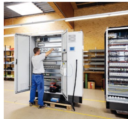
Control cabinet construction in the plant nearby
