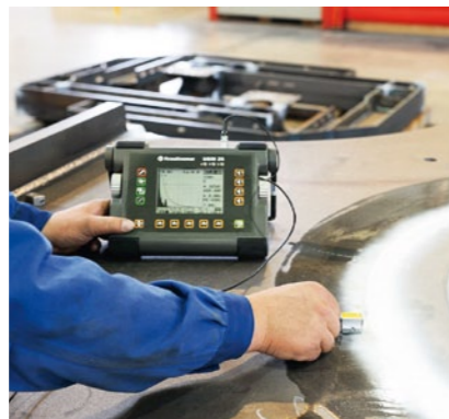
Ultrasonic testing of welded seams
