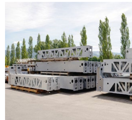
Galvanized stacker crane masts
