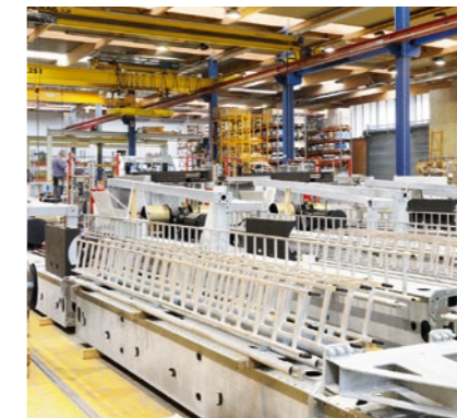
Assembly of the parts on the stacker crane mast
