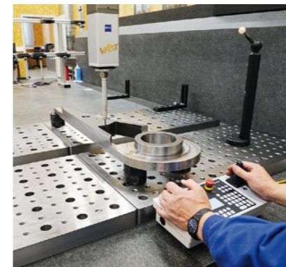
Open test location with Zeiss measuring machine
