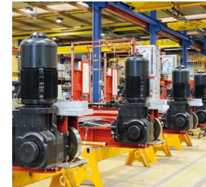
Mechanical assembly of the stacker crane chassis
