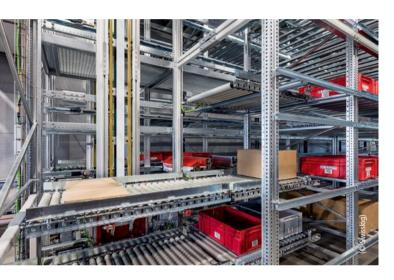
A dynamic double-deck lift transfers cartons and totes pulled by CycloneCarrier shuttles to pick stations or palletizing robots.
