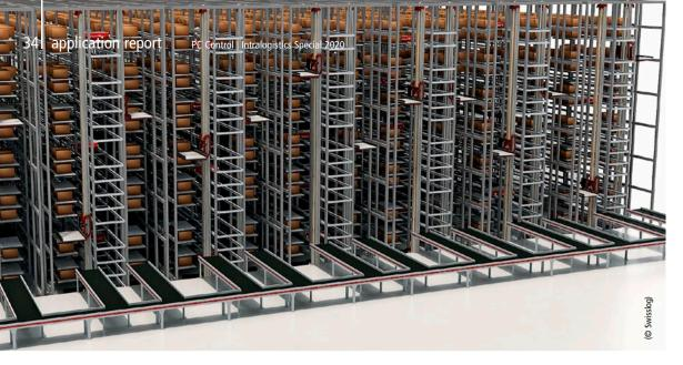
The compact shuttle vehicles travel at speeds up to 4 m/s across the shelving, which offers a maximum footprint of 150 m long and 25 m high.
