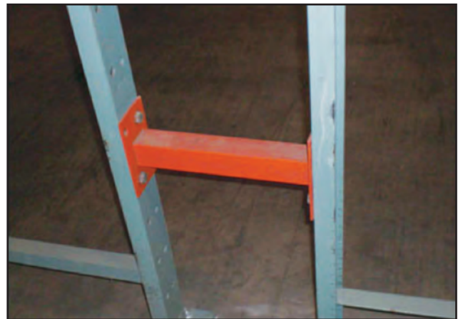
Example of structural row spacer
