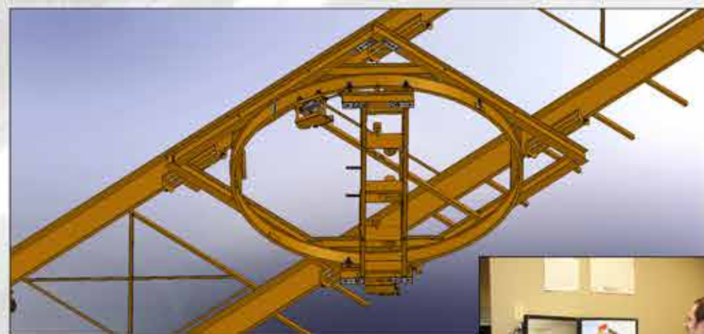
3-D Model of custom designed patented track rotating trolleys
