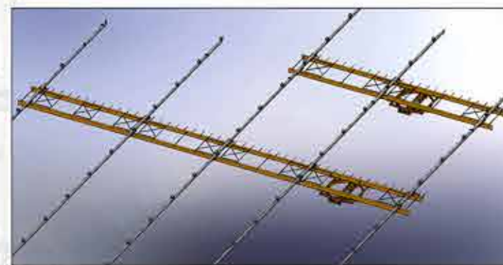
3D layout of double girder multiple runway patented track cranes for an aircraft manufacturing facility
