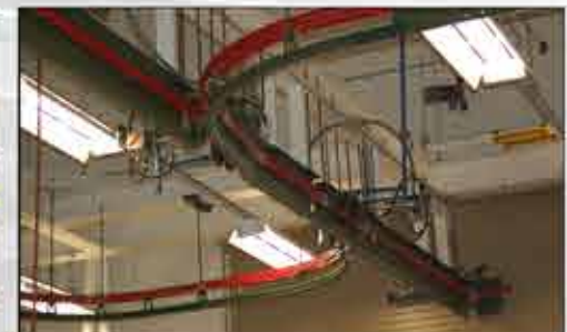
Patented Track Monorail with Switches
