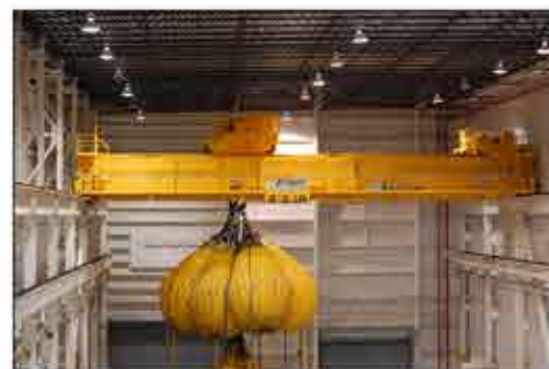
250-Ton Load Test using 625,000 pounds.
