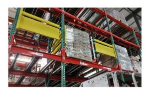
Double width bays have a unique challenge. How to best keep a worker from an exposed fall opening or gap? The Gate arms must maintain the 200lbs load force requirement in the event of a fall. AND...
