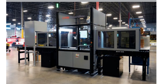
Automatic box-resizing system to reduce parcel shipping costs
