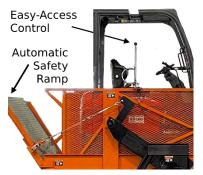
IT'S SAFE: The Speed-Lift is *always* level. The forklift operator can raise and lower the Speed-Lift *without leaving the safety of their seat*. Forward and rear ramps *automatically open and close* to ensure that the operator cannot drive off the end.
