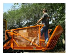
**IT'S VERSATILE**: Unlike a ramp, you can also safely walk on a Speed-Lift with a loaded pallet jack. If you already have a dock, a Speed-Lift can even enhance its functionality. Speed-Lift capacities range from 5000-25000 LB.
