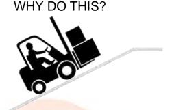
The best way to avoid two of the main causes of overturns is to avoid driving on uneven surfaces or inclines (ie. yard ramps). Keep it level.
