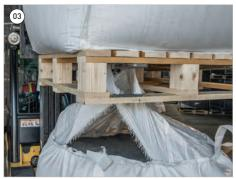
Standard pallets have large openings at the bottom for support which can quickly result in damages to bulk bags.
