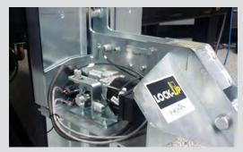
Sealed magnetic proximity sensors with direct drive gear motor
