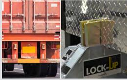
Vertical barrier ensures engagement by securing intermodal container chassis with rear impact guard obstructions
