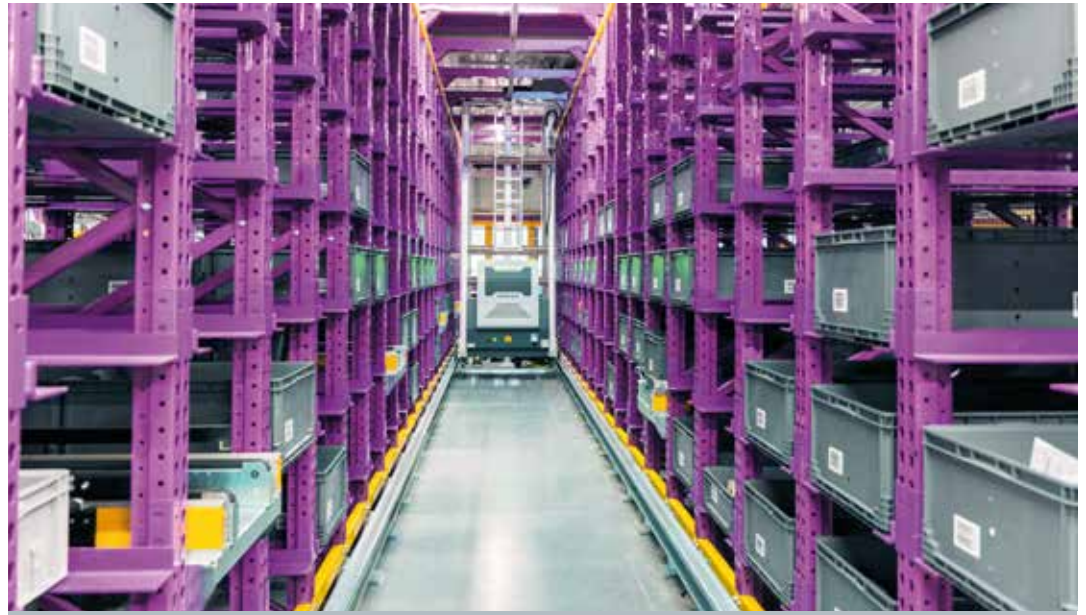
3 | The GEBHARDT StoreBiter® Multi-Level-Shuttle warehouse serves as intermediate storage and packaging of the suspension.
