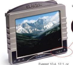
Button Panel left to right: Information LED (N/A), Battery Indicator, HD Access, Power On, Power Button
