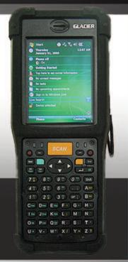
The Glacier M300 offers an innovative, slim design that is super rugged and loaded with the features your mobile workforce requires. The M300 represents a new standard for data collection in harsh environments. Designed and tested to an IP65 rating and drop tested to 6 feet to concrete, the M300 rugged PDT will withstand wet, dusty environments as well as extremes of temperature.
