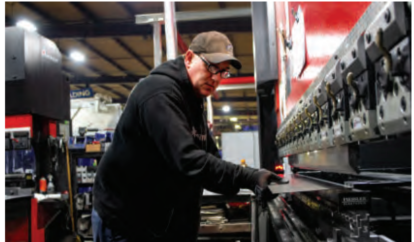
Press brake operator Nick Fay forms a part. The brake is mere steps away from the laser cutting machine's offloading table.
