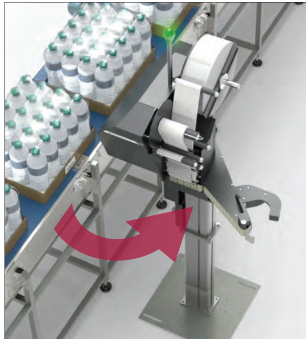
THE 258 ROTATED INTO SERVICE POSITION
