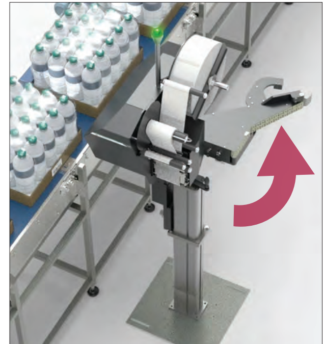
THE CROSSMERGE™ MODULE ROTATES FOR MORE ACCESS
