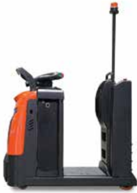
T66N 6,600lb Capacity Rider Electric Tugger Lithium-ion Option Available
