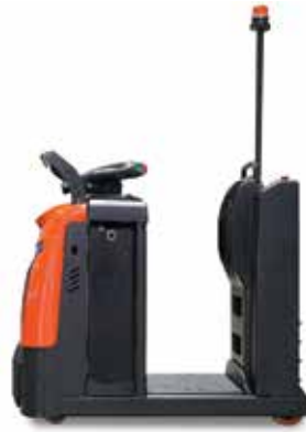
T110N 11,000lb Capacity Rider Electric Tugger Lithium-ion Option Available
