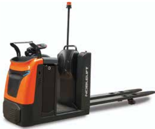
OPL55N 5,500lb Capacity Low-Level Electric Order Picker Lithium-ion Option Available
