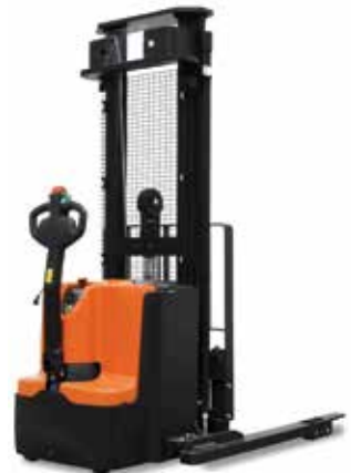
PS35TSL, PS40TSL 3,500 - 4,000lb Capacity Electric Stacker Polyurethane Tires Lithium-ion Option Available
