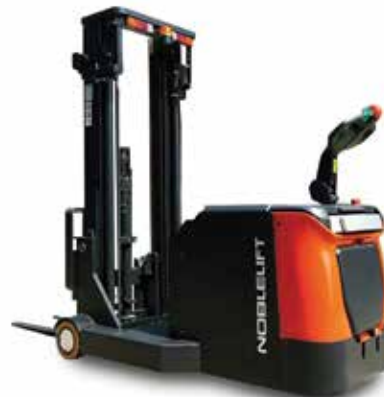
PS20-30-40CB 2,000 - 4,000lb Capacity Electric Counterbalanced Stacker Polyurethane Tires Lithium-ion Option Available
