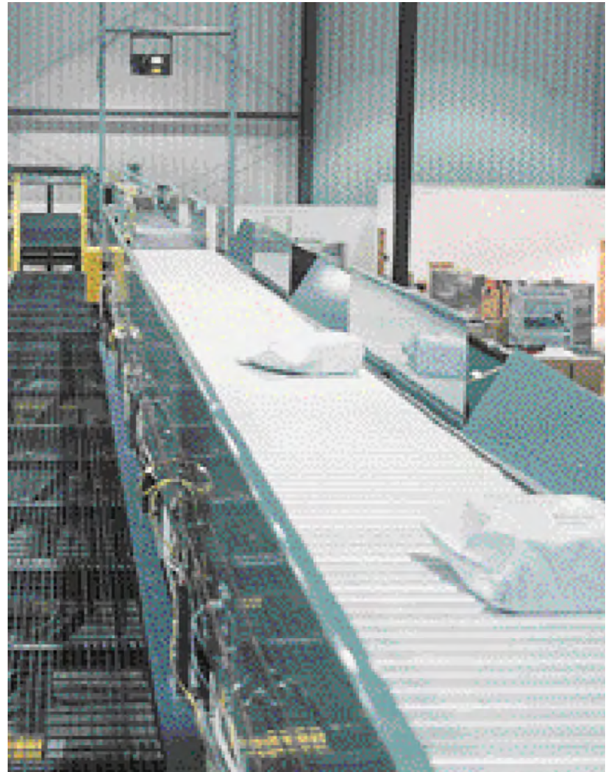
The Hytrol ProSort 100 Shoe Sorter operates at 230 cases per minute and can handle 60,000 packages a day.
