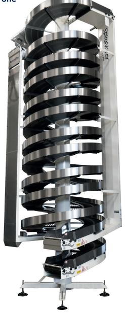
The Nested-configuration is a multi-track spiral that offers the most compact and flexible spiral conveying solution. The Nested-configuration can be applied for both elevation and accumulation purposes. The spiral is based on the idea that you can wind more than one track around the same vertical axle. These tracks can have the same belt width.
