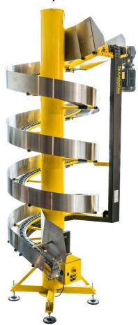
The spiral conveyor specifically designed for jobs like these is the SpiralVeyor® ToteLift. This spiral utilizes a unique belt type that provides a significant amount of added grip on the totes when compared to standard spiral conveyors. By doing so, the totes will not slip even when running at higher speeds, with a small radius, and at steep inclines. This solution will always deliver a controlled flow of items and recovers more than 50% of the space from the old sliding chutes.
