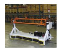
This robust unit is used as a mobile assembly line for dashboards and sub assemblies then also serves as a delivery vehicle to the assembly line of an automobile manufacturer. Each fabricated steel unit is powered by a Creform bolt-on AGV.
