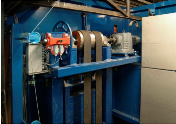
Drive unit with geared motor, coupling, drum and interlock
