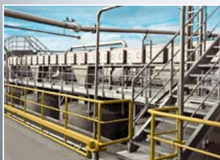
Gas-tight horizontal pendulum bucket conveyor
