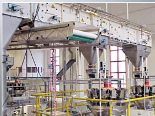
Pendulum bucket conveyors can have any number of discharge points
