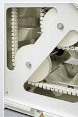
Transition from horizontal to vertical conveying
