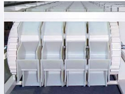
Multiple bucket belt at the tensioning unit
