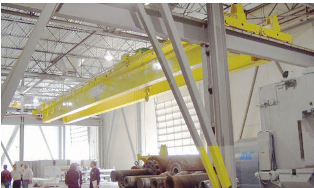
Class D Heavy Use cranes are used in heavy machine shops, foundries, fabricating plants, steel warehouses, container yards or lumber mills.
