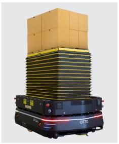
Gross payload without attachments. Maximum payload is 1,500 kg (3,300 lbs.) with hydraulic lift or in-line conveyor attachment options.
