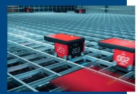
This is in contrast to fixed-shuttle GTPs where storage and throughput capacity are added in tandem. Roaming shuttles help to reduce overall building footprint by taking full advantage of the clear height of the facility. Some roaming shuttle systems are configurable to take advantage of odd-shaped spaces as well. They are gaining traction as part of local or micro-fulfillment solutions. Factors for consideration when evaluating these types of bots include:
