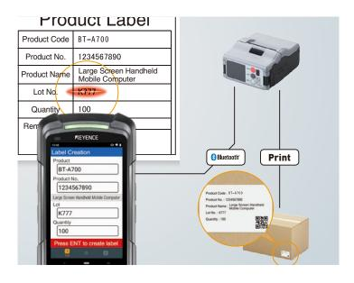
Barcode labels can be printed on the spot for items without barcodes through on-site reading of characters. This reduces the risk of affixing the wrong label and the burden of having to create labels in an office.
