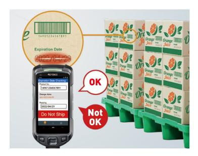
Reading of expiration dates for food products is possible, enabling better management of which products should be used first. This also helps eliminate complaints from shipping destinations by ensuring adequate time before products expire.
