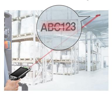
Readers can be used to read nonbarcode characters in location signage. This enables simplified location management using only existing assets.
