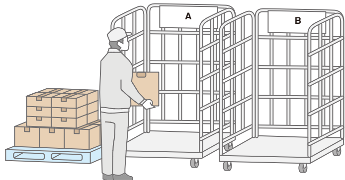
A method in which the necessary quantity of products is gathered per item and sorted by destination.
