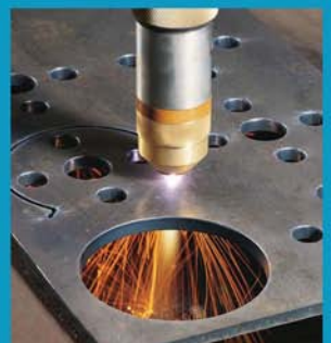
Precision parts cut to .020 tolerances
