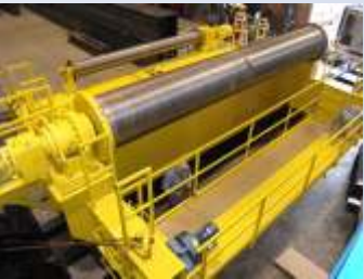
A 250/50 ton engineered crane undergoes load testing at a power plant. The specially engineered hoist at right features a service walkway to facilitate maintenance.
