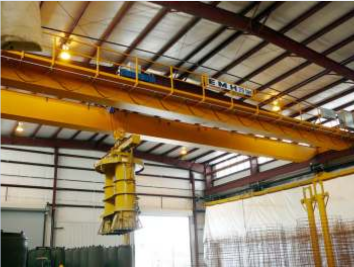
EMH is experienced in building cranes for the concrete industry. The crane at left is used with a Hawkeye machine by a manufacturer of concrete pipe.
