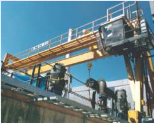
A 25 ton, 120 foot gantry (above) positions architectural concrete panels on trucks for shipment.
