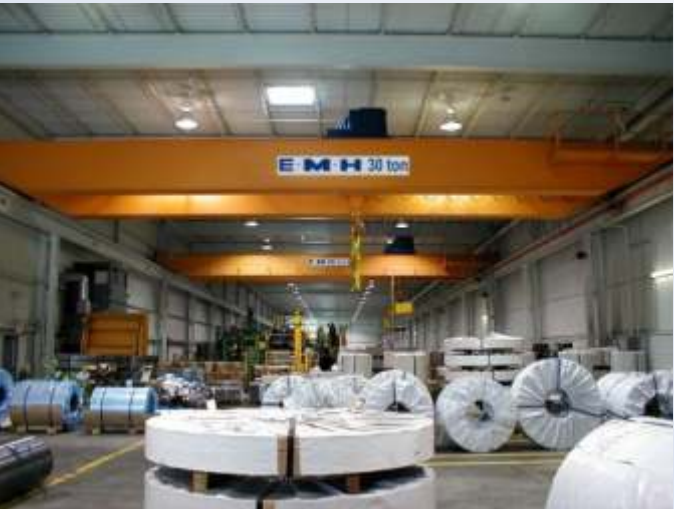
Two 30 ton EMH cranes with engineered hoists move large coils for two shifts each day at an Ohio steel service center.
