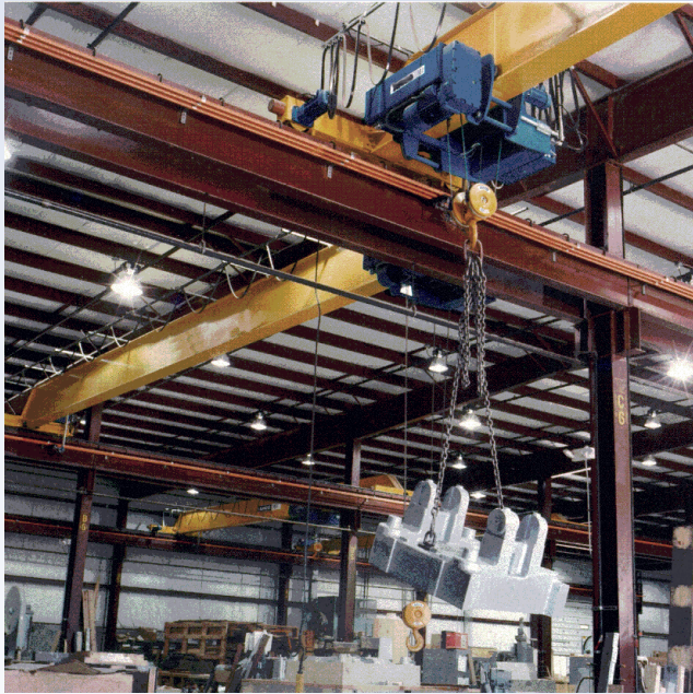
Four single girder cranes in a mold pattern shop.
