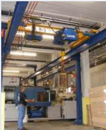
A NOMAD System at a Midwestern manufacturer of industrial containers was installed on a 182 foot freestanding runway located between concrete building supports.
