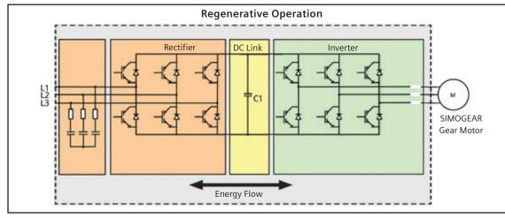
By using an IGBT front-end instead of the rectifier circuit found in most drives, the Siemens G120D distributed drive recovers energy generated by high-inertia loads and places it back onto the incoming line. This saves energy, simplifies the design and installation, and saves costs.
