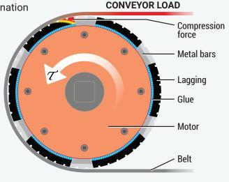
This revolutionary design significantly reduces wear, maximizing conveyor system life and minimizing maintenance.
