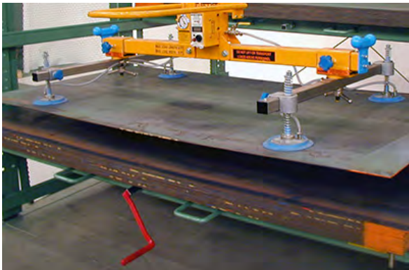
A vacuum lifter retrieves an individual sheet out of a Crank-Out Sheet Rack Drawer
