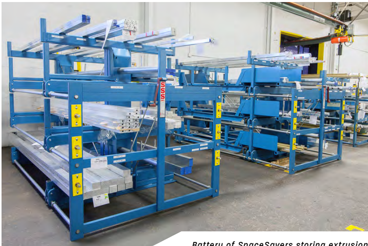
Battery of SpaceSavers storing extrusion
