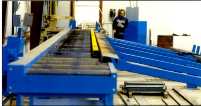
Pushbar ejecting material onto discharge skids.
