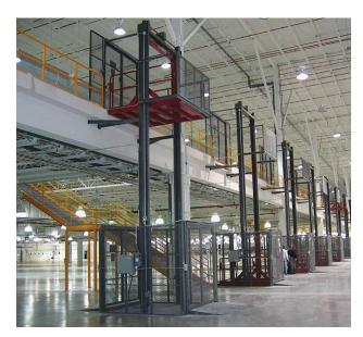
With carriages designed to accommodate a company's exact specifications, VRCs take up a relatively small amount of space when compared to other forms of product transportation. This benefits a facility's overall floorplan by maximizing the available square footage. Additionally, VRCs are traditionally installed near key product storage and transportation points. This reduces the number of times a product is handled, allowing employees to concentrate of more critical operational activities.
